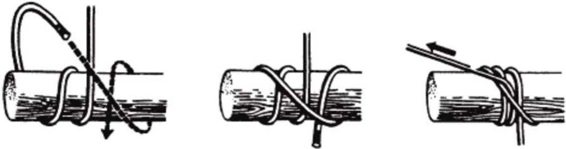
Figure 15D-1 Steps to Tying a Rolling Hitch
