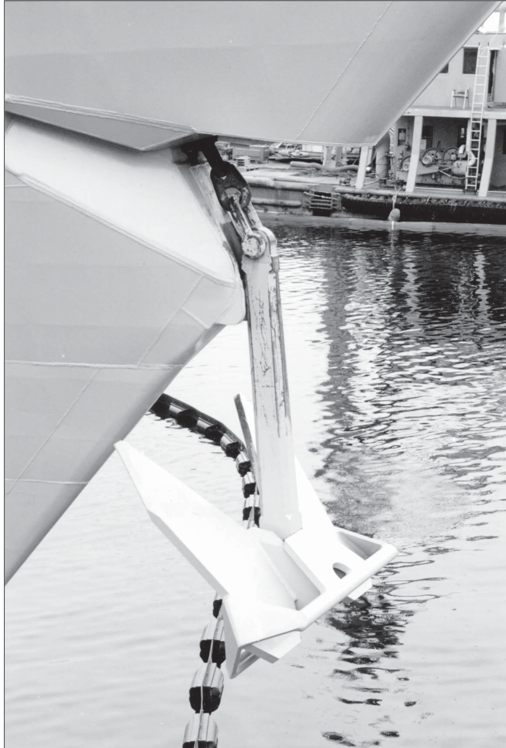
Figure 7.6-3 - HALIFAX Class Pool KM 2835 kg
