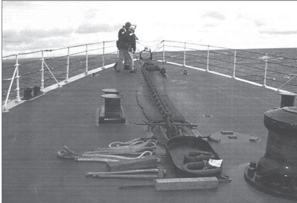
Figure 8.12-2 - Towing Receive Forward Layout
