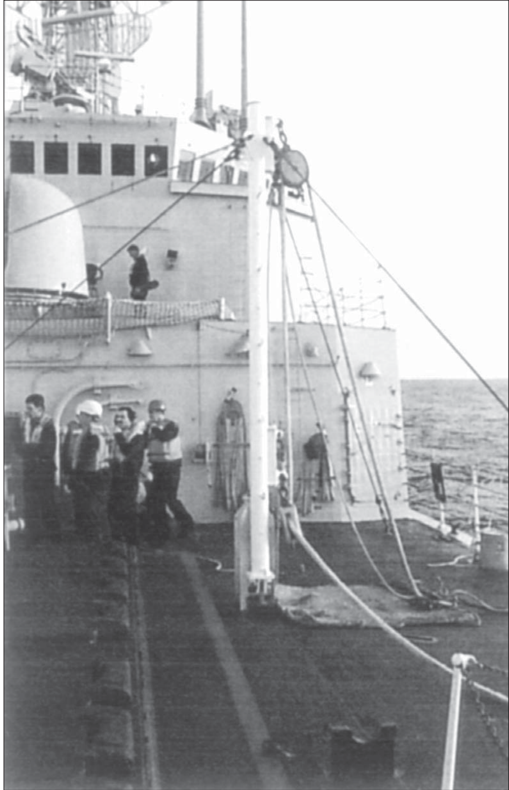
Figure 9.21-2 - Light Jackstay Supply Port (Looking Aft)
