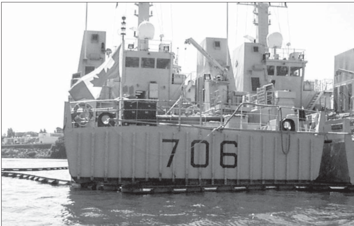
Figure 8.14-11 - Stern View of Towing Pennant, Towing Hawser & Recovery Line (lashed to guard rail) KINGSTON CLASS
