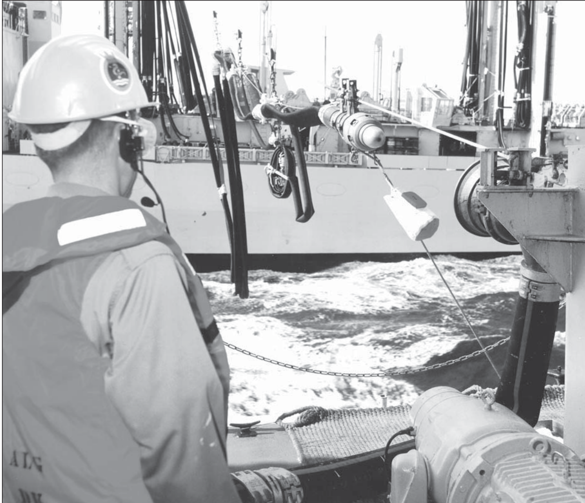
Figure 9.14-1 - Probe Fuelling AOR 509/510 and IROQUOIS Class
