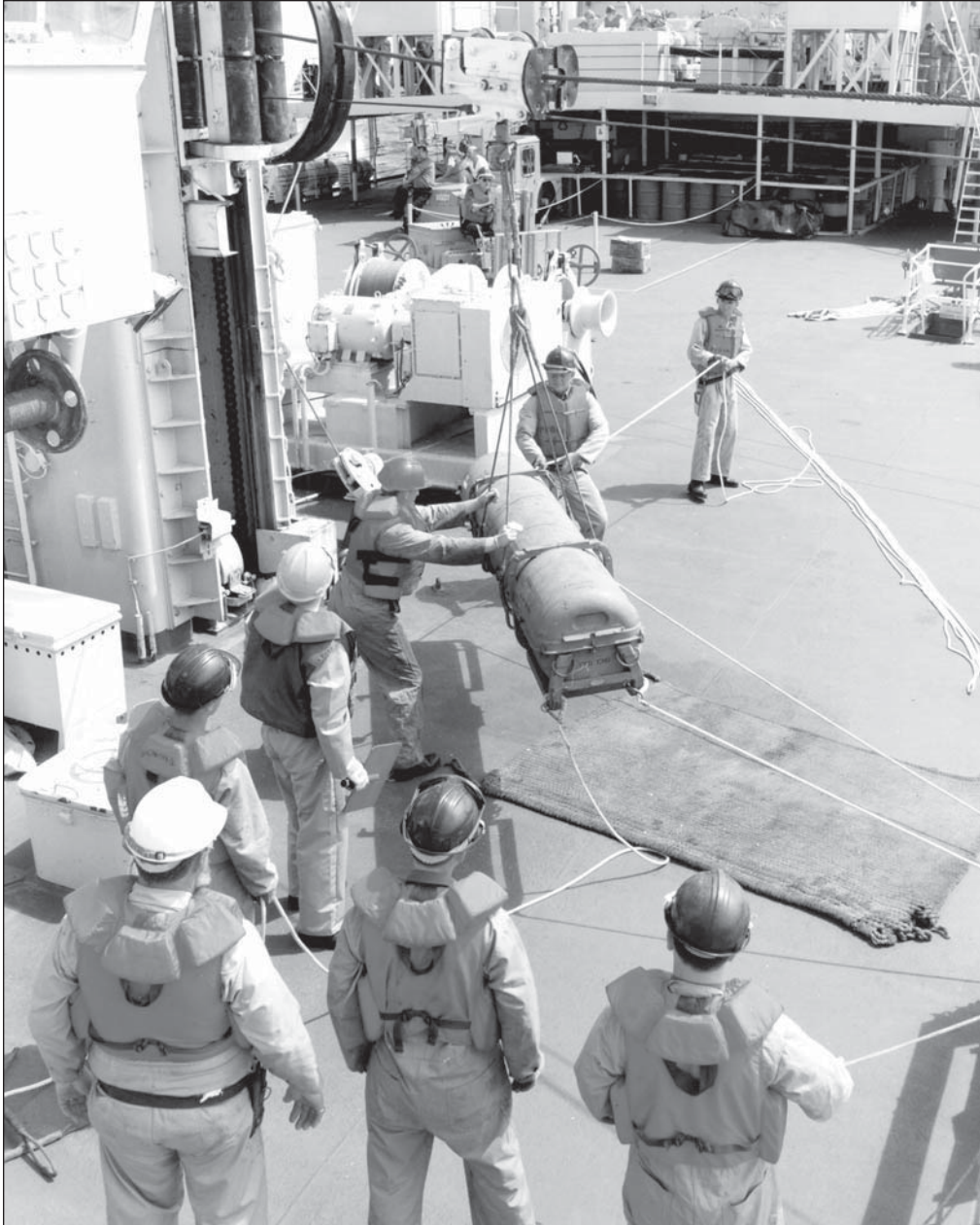
Figure 9.13-2 - Torpedo Transfer Heavy Jackstay
