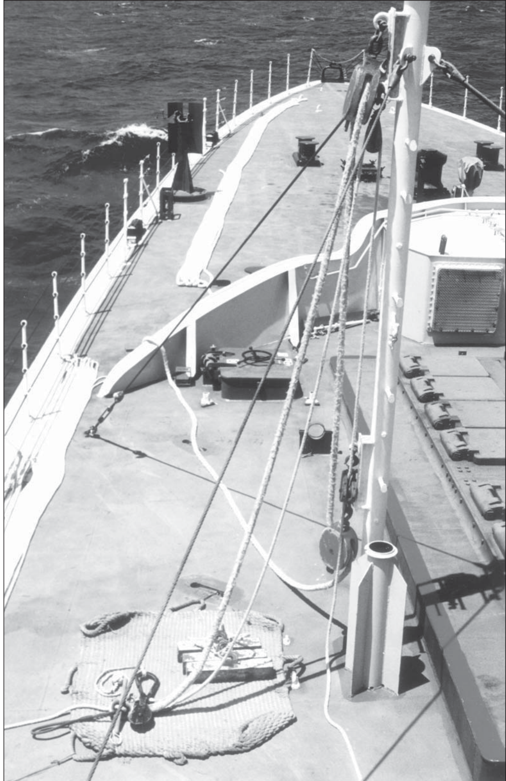
Figure 9.21-3 - Light Jackstay Supply Port (Looking Forward)
