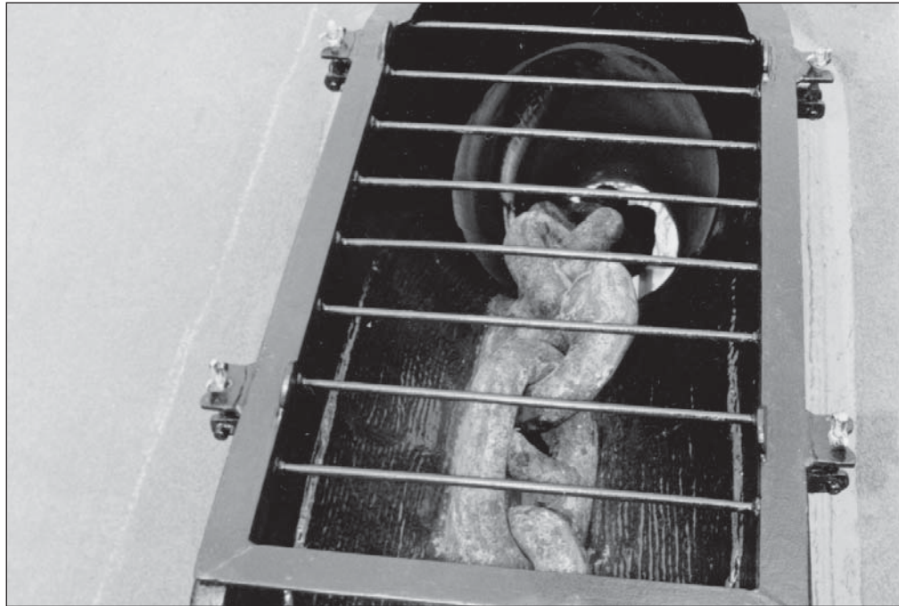
Figure 7.4-3 - Hawse Pipe with Deck Bolster
