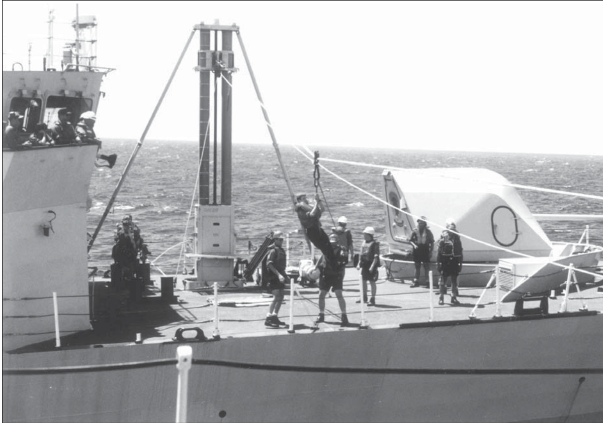
Figure 9.22-9 - Light Jackstay Receive Station 1
