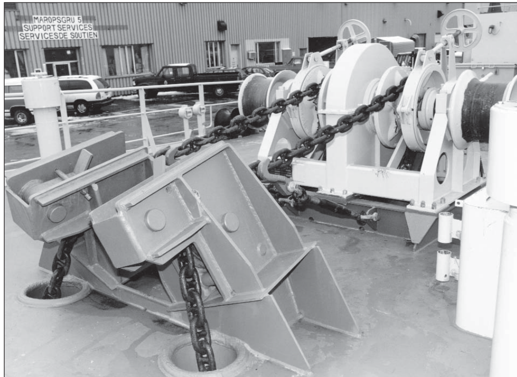
Figure 7.16-1 – Anchor and Cable Arrangements – KINGSTON Class
