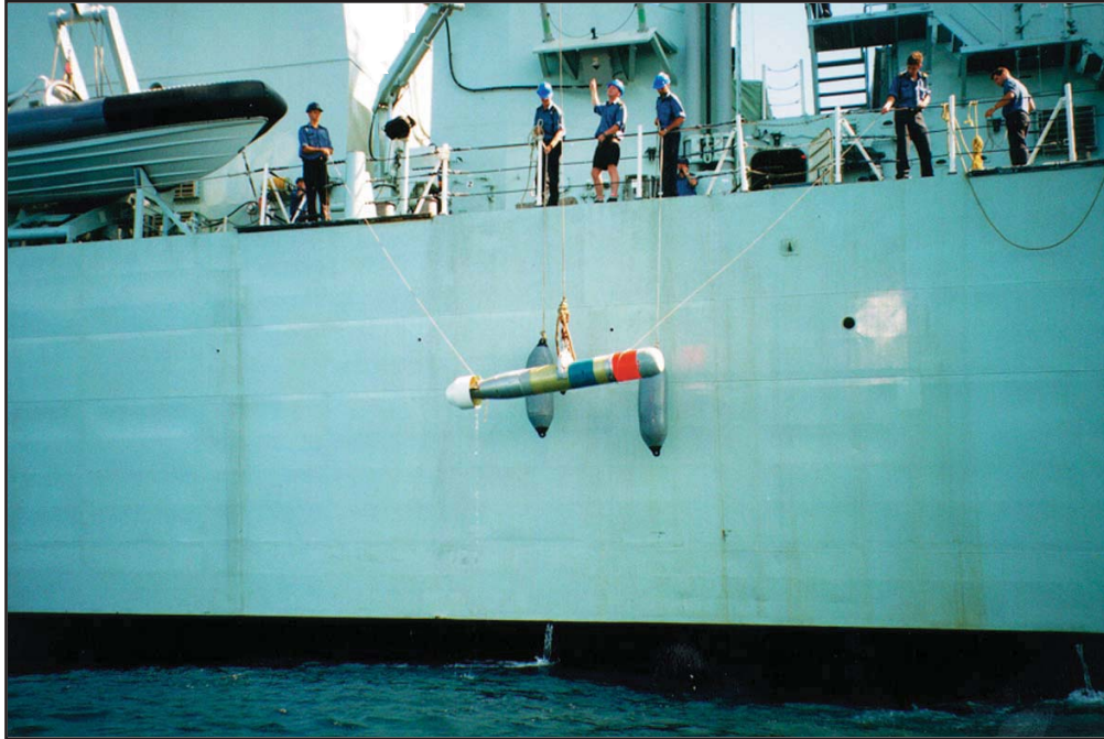
Figure 10.17-2 - Fenders Placed between the Ship and Torpedo
