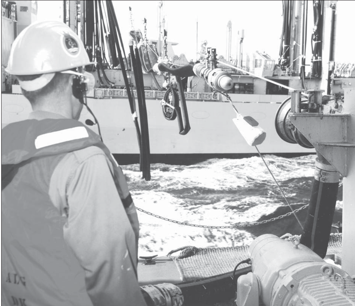
Figure 9.23-6 - Probe Fuelling AOR 509/510 and IROQUOIS Class
