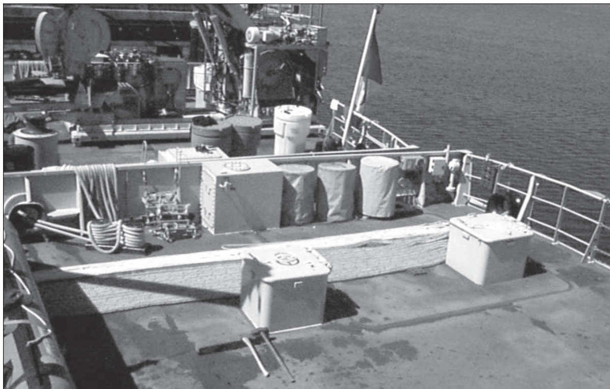
Figure 8.14-13 - Sweep Deck View of Towing Lay out KINGSTON CLASS
