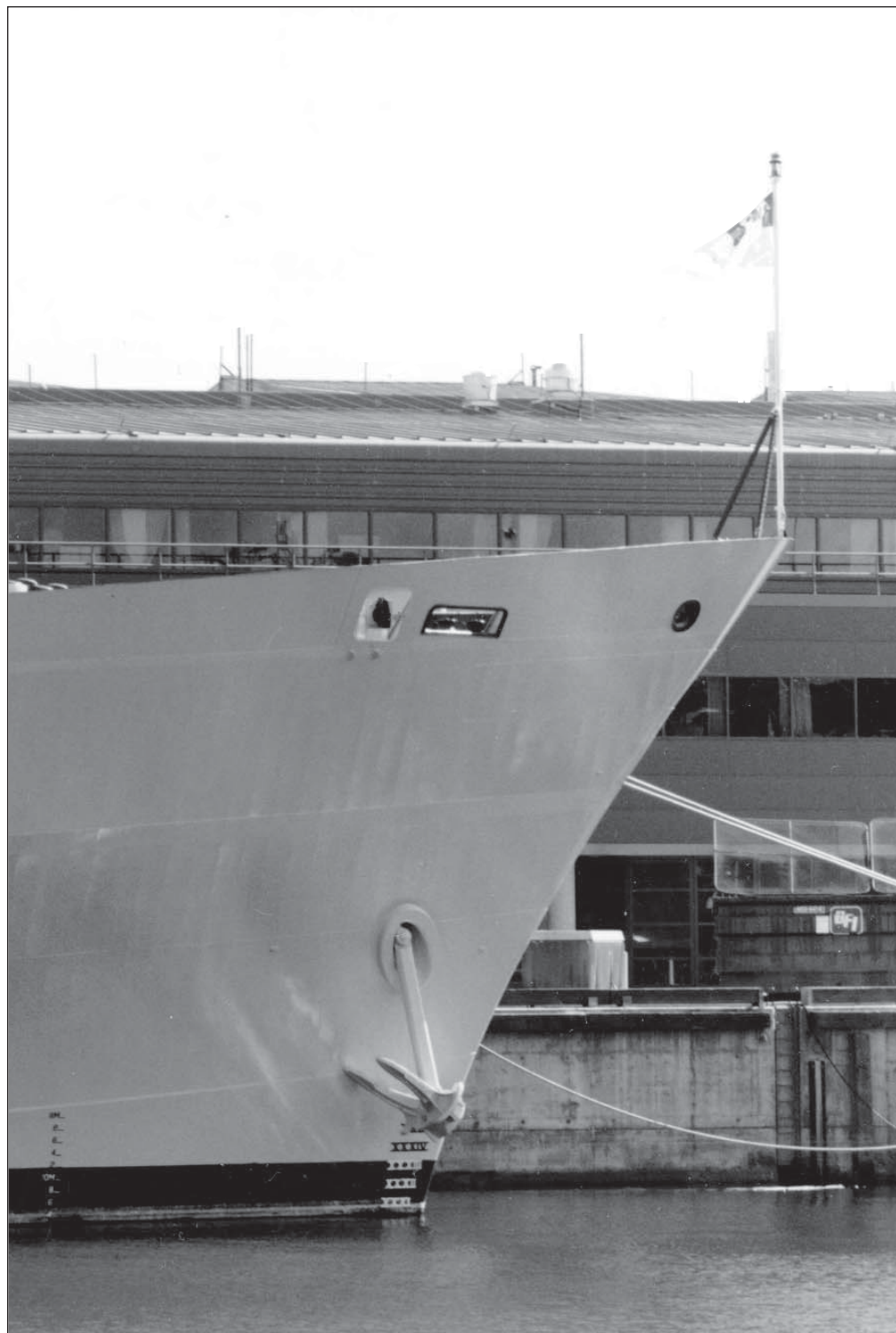
Figure 7.6-6 - AOR 509 Class Marine Fluked Stockless 5448 kg
