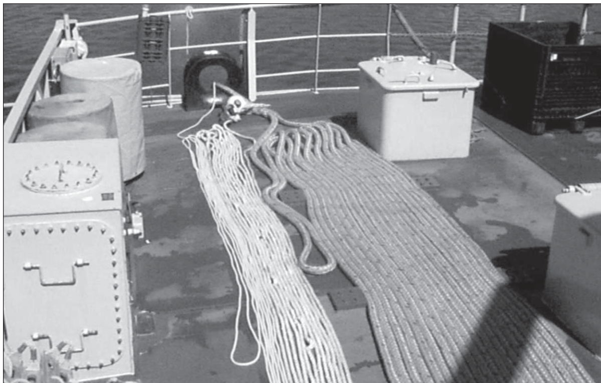
Figure 8.14-7 - Towing Lay Out Supply Aft KINGSTON CLASS
