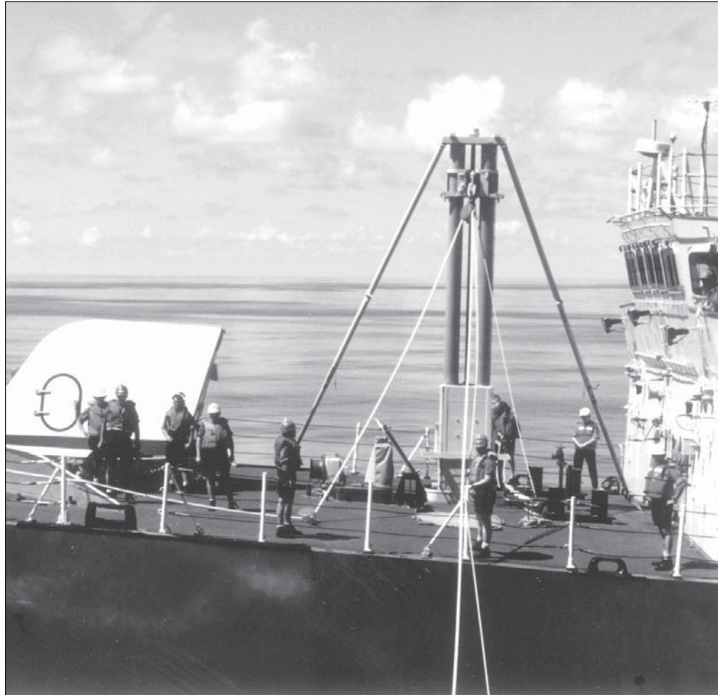
Figure 9.22-3 - Light Jackstay Supply Station 1
