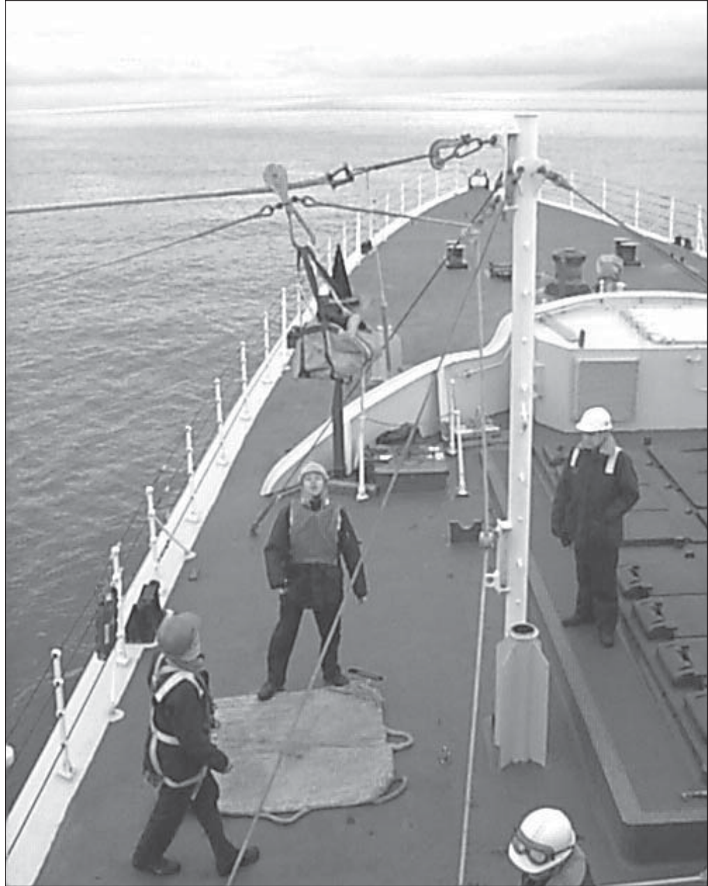
Figure 9.21-5 - Light Jackstay Receive Port
